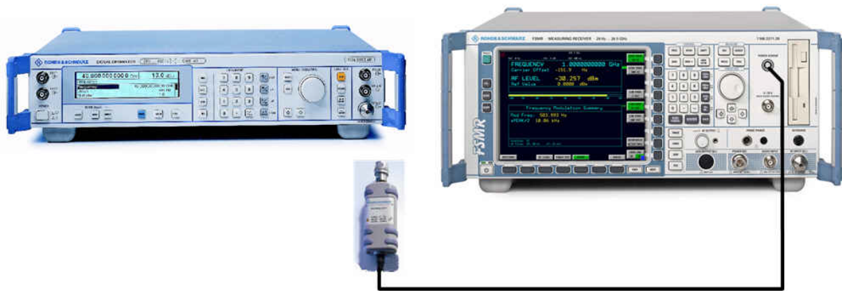
Fig.2-2 RF Power measurement setup
