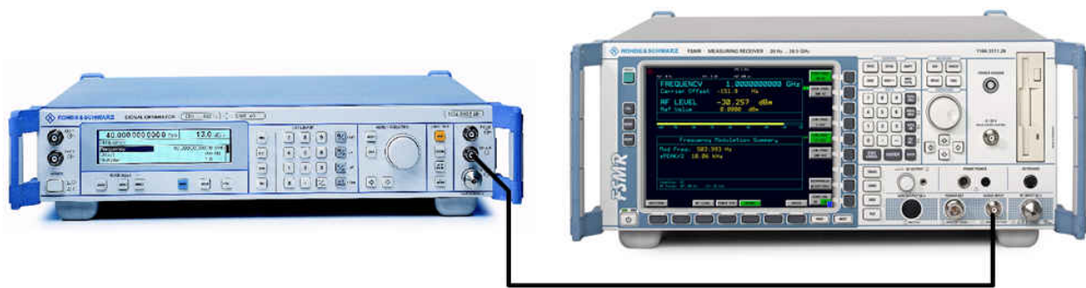
Fig.2-13 Audio measurement setup
