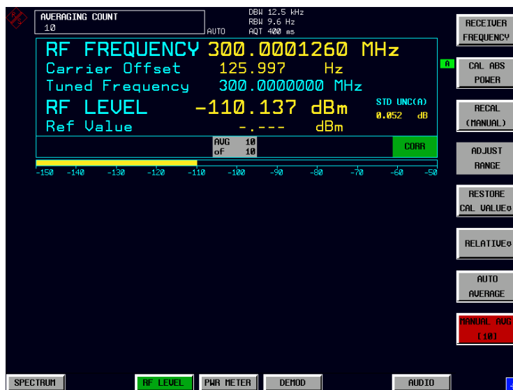
Fig.2-8 Tuned RF Level measurement with Averaging
