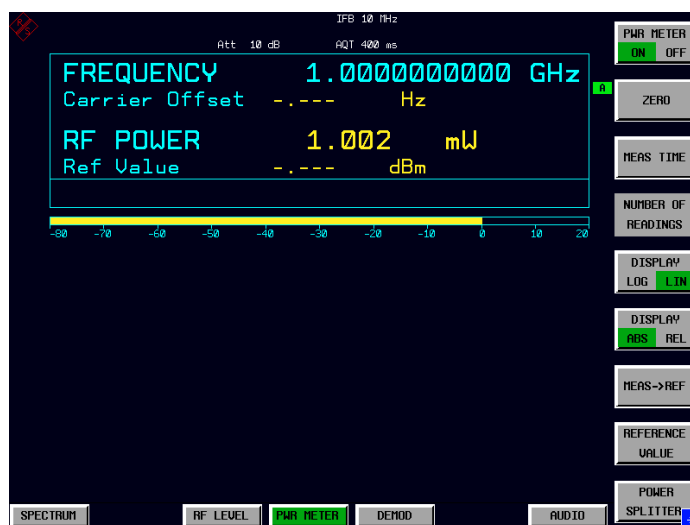
Fig.2-4 RF power measurement in UNIT Watt
