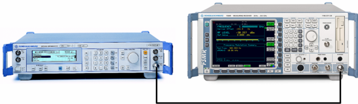
Fig.2-9 AM modulation measurement setup
