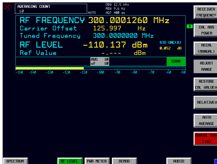
Fig.2-7 Tuned RF Level measurement at low levels
